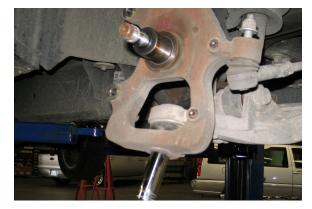
17. After both ball joints are dislodged, remove the upper ball joint nut and lift the upper control arm to free the spindle. Remove the lower ball joint nut and slide the spindle off the lower ball joint.
