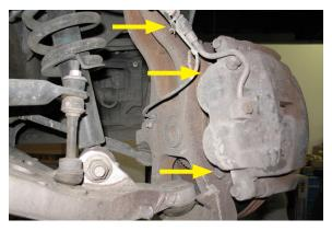
10. Remove the hub and rotor assembly from the spindle by removing the cotter pin, retainer cap, and the 36mm spindle nut from the spindle pin. Slide the rotor assembly off the spindle pin and set it aside
