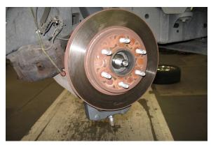
25. Torque to spindle nut to 295 ft lbs. Insert the supplied cotter pin into the hole in the spindle pin. Bend the ends of the cotter pin against the nut and cut them off. Place the retainer cap over the spindle nut.
