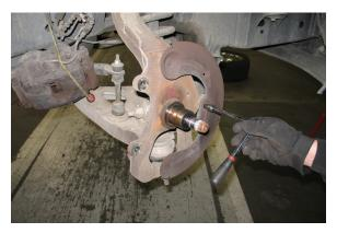
12. Remove the 8mm bolt from the wheel sensor at the steering spindle. Detach the clip holding the sensor line to the upper control arm. Place the sensor away from the work space.
