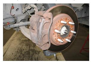
27. Rotate the spindle assembly in both directions to confirm if the brake line and sensor cable have proper clearance. If needed, adjust as necessary.
