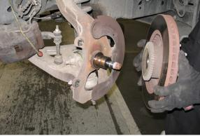
11. Remove the three 8mm bolts from the dust shield and detach it from the face of the spindle.
